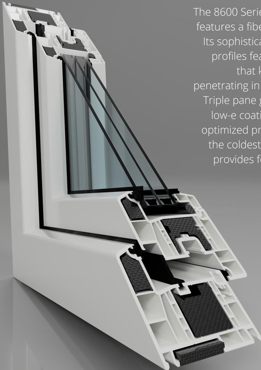
The 8600 Series of windows and doors features a fiberglass core for strength. Its sophisticated six-chamber, 86mm profiles feature a triple seal system that keeps water and air from penetrating in the harshest conditions. Triple pane glazing with two layers of low-e coatings along with thermally optimized profiles keep you warm on the coldest days. Roto NT hardware provides for high security and high structural performance.
